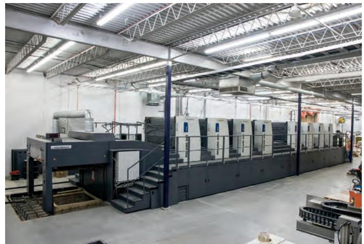
The press is being installed and should be running colour signatures mid to late May.
